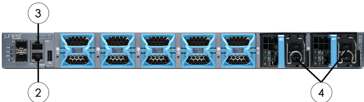
Figure 9. Juniper QFX5200-32C high-bandwidth Ethernet data switch (rear view)
